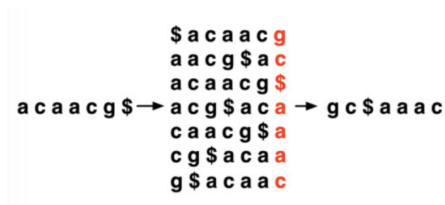
Figure 5: Example of the Burrows-Wheeler Transform ($ represents the end character)
